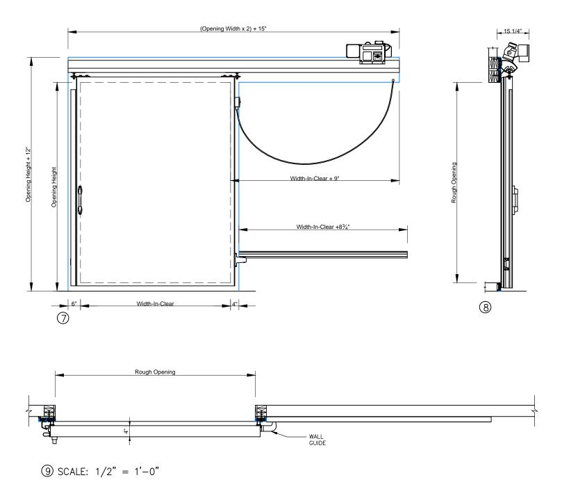
Page 3/4 Single Horizontal Electric Slide Door with Backup Casings and Return Jambs Model EFD-SHES (7) ELEVATION - HIGH SILL SLIDING DOOR (EXTERIOR) Wall Guide SECTION - HIGH SILL SLIDING DOOR Exterior Pull Handle with Interior Recessed Handle (9) JAMB - HIGH SILL SLIDING DOOR
